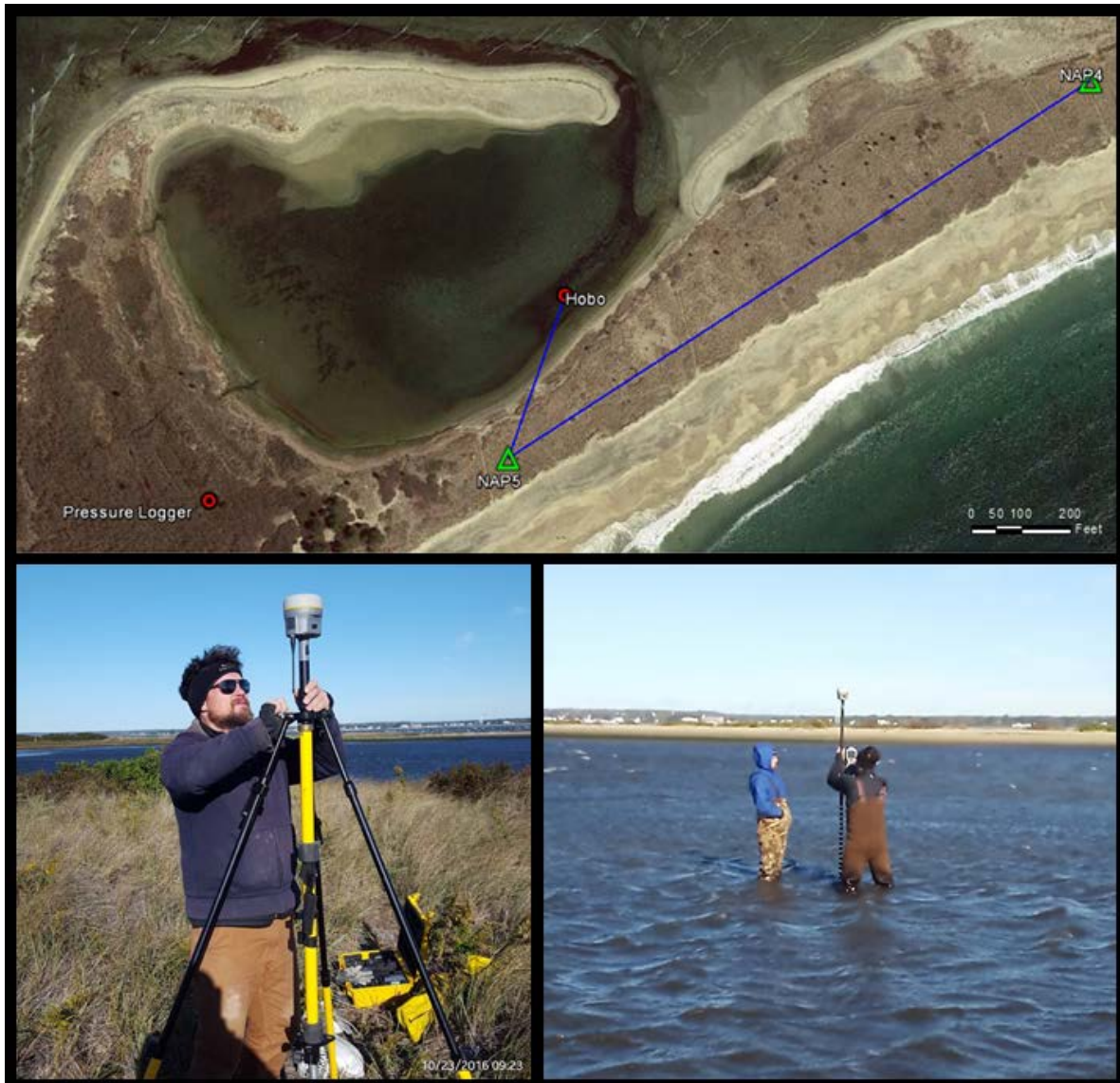
Figure 1. Top: location of water level logger, atmospheric pressure logger, RTK-GPS base receiver, and survey check-in location. Blue lines represent RTK baselines from the base receiver to the rover receiver. Bottom left: RTK-GPS base station set-up. Bottom right: Hobo survey.
